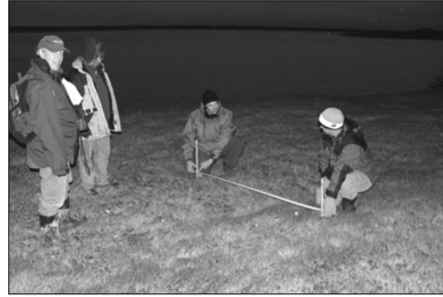
Setting up of monitoring point for frost cracks near the riverbank, involving a metal pin on each side of the crack and measurement. (K. Skaftfeld)
