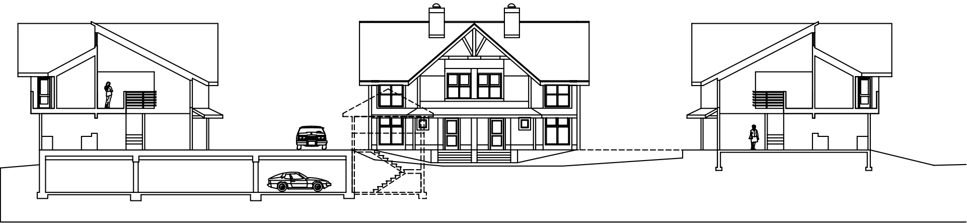
CONCEPTUAL DESIGN - Section across courtyard of building complex showing underground parking
