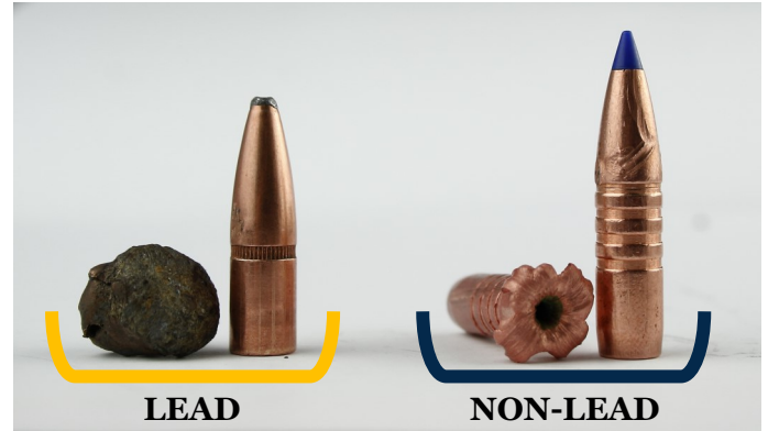
Above: Unspent and spent bullets recovered from harvested moose. The lead bullet has lost most of its lead core whereas the solid copper bullet remained intact. (Photo: Parks Canada)
