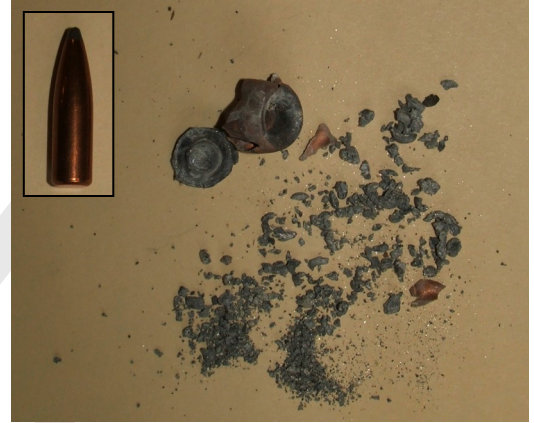
A lead cored bullet before (inset) and after being shot. The lead core has separated and fragmented into hundreds of pieces.
