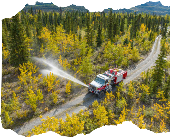
YWFM pumper truck wetting down adjacent fuel.
